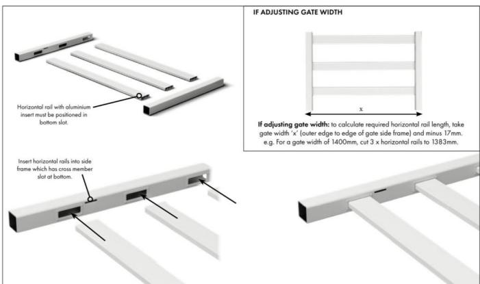
Lay out side frames and horizontal rails on a flat bench.
