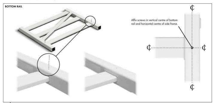
Ensure gate square. TIP – measure diagonals ensuring the same measurement.
