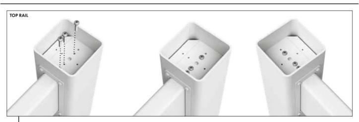
Screw top rail into place inside side frame using 3 x 25mm screws.
