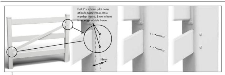
The cross member must be fixed off at both ends. Drill 2.5mm pilot holes 8mm in from edge of gate side frame. Fix off at bottom and top side of cross member using 2 x 50mm screws.
