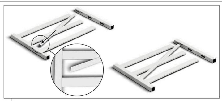
Insert cross member into the gate side frame at bottom side (same side frame that horizontal rails have already been inserted).
