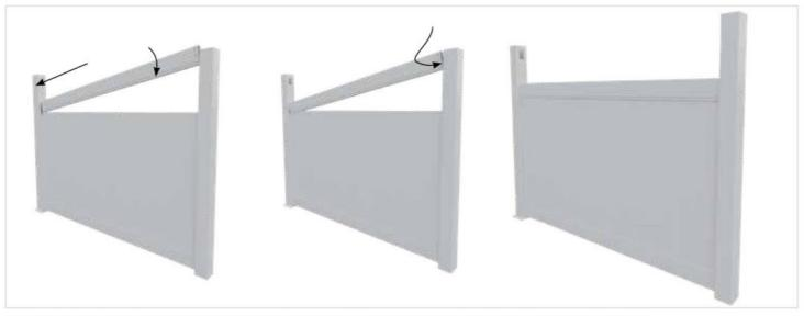
Install mid rail over vertical panels and simultaneously push top rail as far as possible into one post and then slide back into adjacent post.
