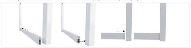
8 Slide bottom rail with aluminium insert into first post as far as possible and lever into adjacent post. Slide back bottom rail to ensure notches have passed into adjacent post.
