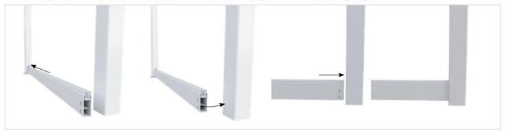
8 Slide bottom rail with aluminium insert into first post as far as possible and lever into adjacent post. Slide back bottom rail to ensure notches have passed into adjacent post.
