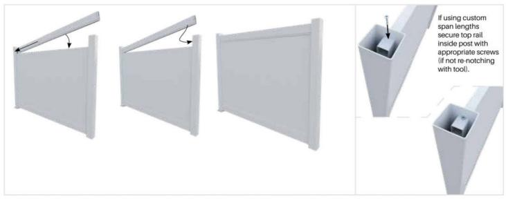
Install top rail over vertical panels and simultaneously push top rail as far as possible into one post and then slide back into adjacent post.
