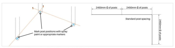
Mark post to post centres using appropriate markings such as spray paint or stakes. Standard fence panel post centres are at 2450mm. If using shorter spans, space posts appropriately. Posts are 127x127mm square.
