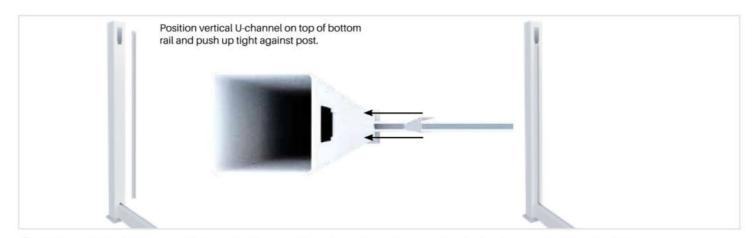
9 Position vertical U-channel on top of bottom rail and push up tight against post. Repeat step on all posts, where fence panels are to be installed. U channel will be held against post both sides once vertical panels installed (no fixing required).
