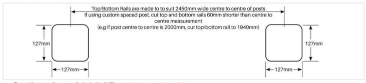
Top and bottom rails are supplied suited to 2450mm centre to centre post spacing.
