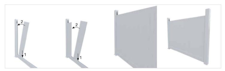
10 Starting at the vertical U channel on one side, insert vertical panels into bottom rail and lever into position. Repeat process towards the next post. If using a custom length span, the last vertical panel will required cutting to size. Refer next step.
