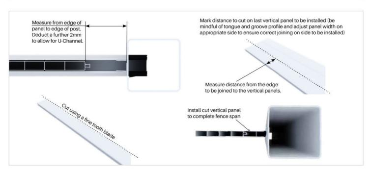
The last vertical panel in the span may need cutting to fit. Mark distance to cut on last vertical panel to be installed (be mindful of tongue and groove profile and adjust panel width on appropriate side to ensure correct joining on side to be installed) and cut using a fine tooth blade. Follow manufacturer's instructions for safe use of saw.
