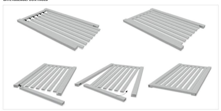
Insert palings into bottom rail. NOTE: Palings have a notch on one end – use notched end as BOTTOM of paling. When a Midrail is being used, spread both side frames and install the Top Rail into palings one-by-one. Once palings are installed into the Top Rail, slide both side frames into position, engaging the Midrail and Top Rail.
